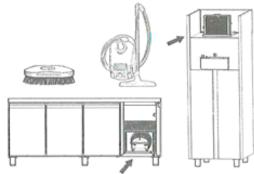
The refrigerated counters with a sliding panel compressor type MG have a filter that protects the condenser from dust, but the filter should be removed and cleaned regularly.
