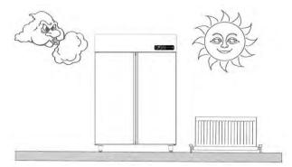
The engine side and mainly the condensing unit must be free from anything that could obstruct good circulation of air around it, even temporarily, otherwise its operation and that of the appliance could be jeopardized.
