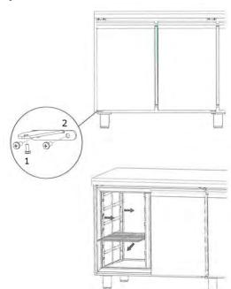
Remove all plastic that supports the metal structure and the plastic that covers the slide guides inputs.
